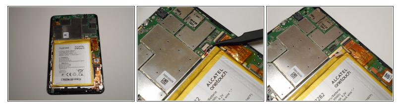
• With the back cover removed you will now want to disconnect the battery. Use the tweezers and gently pull the wires as shown in the second picture.
