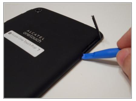
Begin working by using the plastic opening tool to remove the back cover of your Alcatel One Touch Pop 7. Opening the flap as shown in the picture will give you an easier start.
