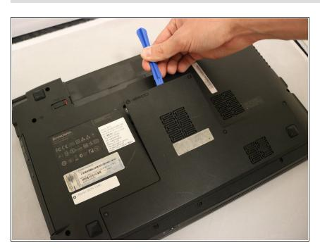
Using a plastic opening tool, pry the back panel from the laptop.
