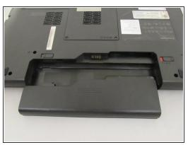
While holding the battery, use your other hand to push the left clip to the left and pull the battery out.
