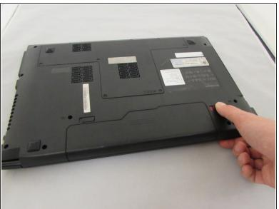
Push the right-hand switch outward into the "unlocked" position.
