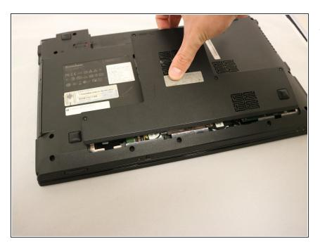
Pull the panel outward from the rest of the laptop. The inside of the laptop will be exposed. From here you can access the CD-ROM drive, hard drive, and Keyboard.
