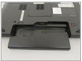
While holding the battery, use your other hand to push the left clip to the left and pull the battery out.
