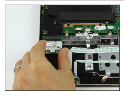
Remove the WLAN chip by pulling out parallel to the surface.
