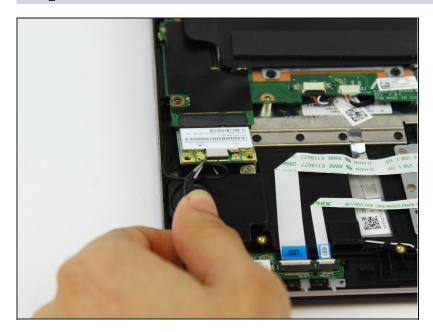
Remove the cable by lifting upwards with a pair of tweezers.
