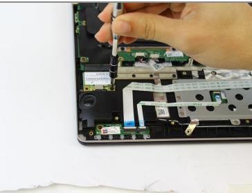
• Remove one 5mm screw using a PH0 Philips screwdriver.
