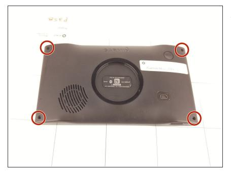
Remove the four, 4mm hex screws at the four corners of the device using a T5 bit.
