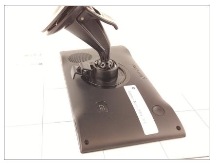
Begin by removing the stand by depressing the tab and rocking the round interface back toward you, pulling it away from the Garmin unit.
