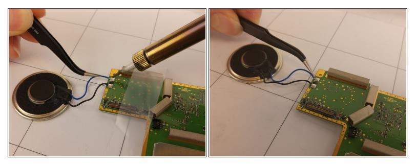
Melt and separate the two metal connections on the circuit using a soldering iron then remove the wires using tweezers.
