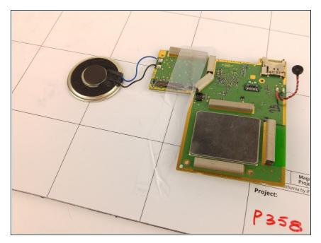
• Tape the main circuit board onto a clean surface to steady the device.
