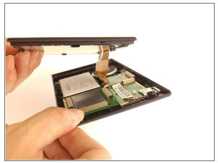
Do not attempt to separate the unit until all the tabs have been separated. Once the seam is completely separated, you can lift the back away from the screen easily.
