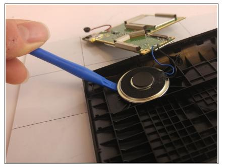
Remove the speaker - located on the device as shown - from the plastic casing using a prying tool. Use the prying tool around the entire rim of the speaker to ensure a clean removal.
