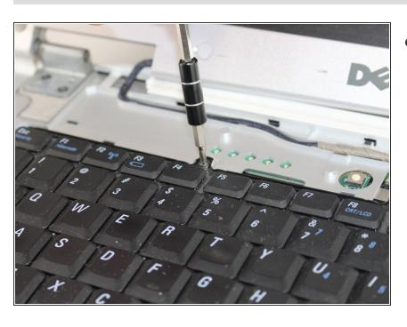
Remove the two 5mm Phillips screws holding the keyboard in place.
