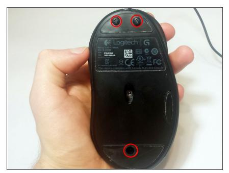
Use a Phillips #1 screwdriver to remove the three 5 mm Philips screws on the bottom surface.
