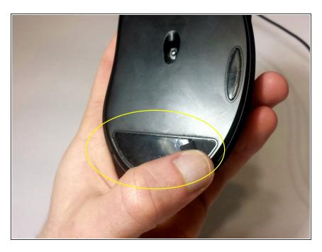
Remove the bottom mouse foot using a Jimmy and the same technique as in Step 1.
