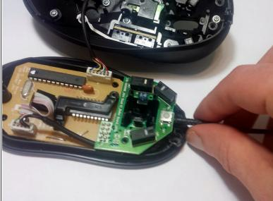
Push the cable into its proper place inside the mouse shell.
