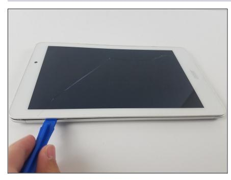
• Wedge the plastic opening tool in between the display screen and back panel
