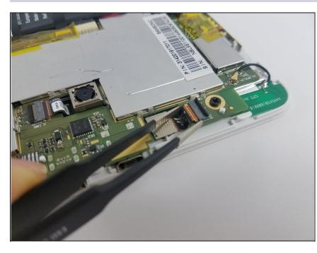
• Use the ESD safe precision <u>tweezers</u> to pull the connector out and carefully remove the camera.
