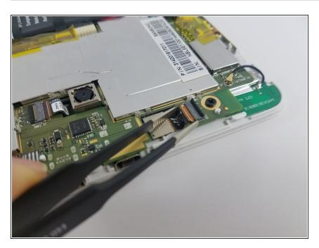
Use the ESD safe precision tweezers to pull the connector out and carefully remove the camera.
