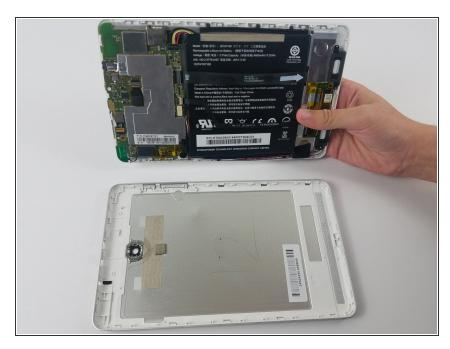
Carefully separate the display from the back panel
