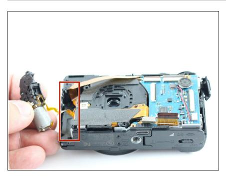
Remove the lens motor by pulling it out of the marked compartment using your fingers. The motor does not have to be disconnected.
