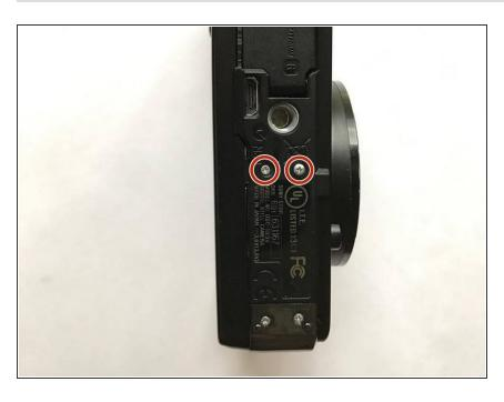
In addition, remove the two marked screws with a Phillips #000 screwdriver.
