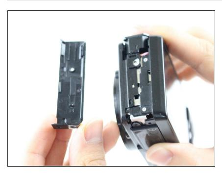
Slide the side cover downward once all screws are removed and place it to the side.
