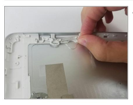
Remove the buttons from the back panel using your fingers.
