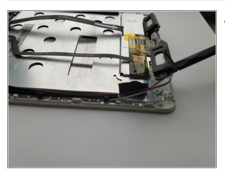
Remove the speakers after unscrewing the screws.
