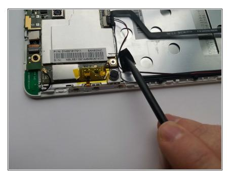
Use the pointy end of the spudger to remove the black tape holding the wires in place and completely free the wires.
