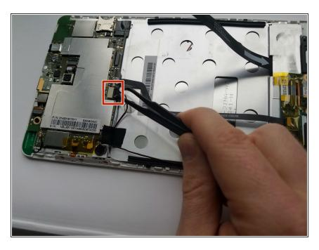
Use tweezers or the flat end of the spudger to carefully pull the connection loose.
