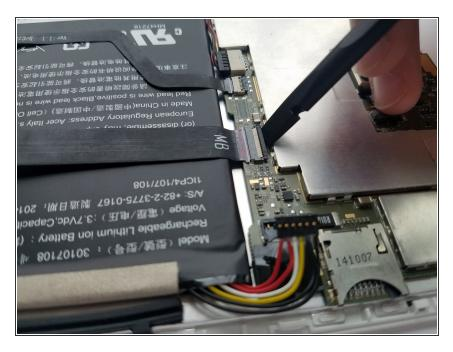
Use the flat side of the heavy duty spudger to lift the small black plastic flap.
