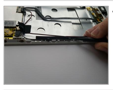
Use spudger to loosen the wire and free the speaker.
