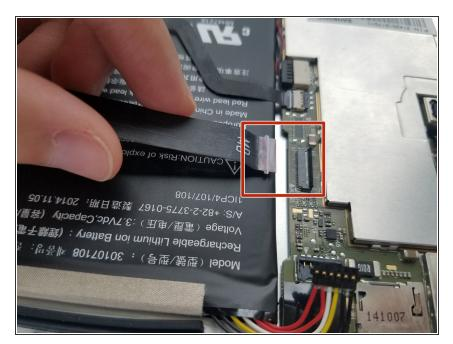
Use fingers to pull the Zero Insertion Force (ZIF) cable from the motherboard.
