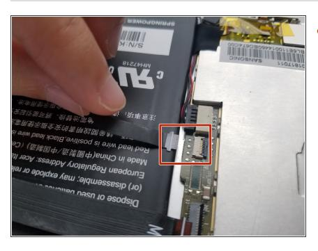
Use fingers to remove the smaller adjacent ZIF cable from the motherboard.
