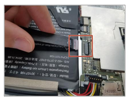
Use fingers to pull the Zero Insertion Force (ZIF) cable from the motherboard.
