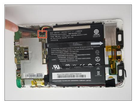
Use the flat end of the spudger to pry up and remove the battery cable.
