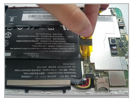
Use your fingers to pull back and remove the yellow plastic tape covering the battery cable.
