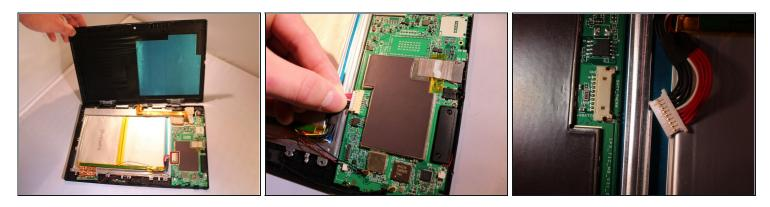
Remove the electrical connector that connects to the battery to remove the power to the battery.
