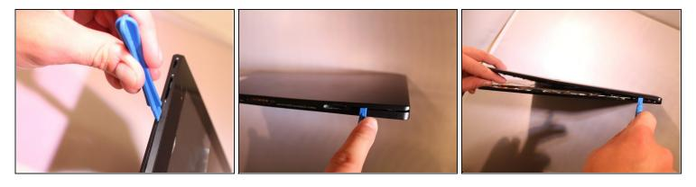
Using a plastic opening tool, gently pry off the back cover.
