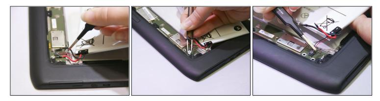
• Pull up the battery cables and battery chip with <u>tweezers</u>.
