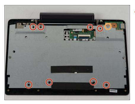
Unscrew the screws on the base plate of the keyboard dock. There should be four 4mm screws along the bottom and four 6mm screws along the top, apart from a single 4mm screw (annotated in orange)
