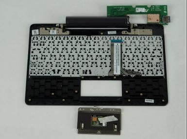
Unscrew three 4mm screws holding the trackpad in place and remove the trackpad.
