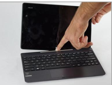
Detach and separate the screen from the keyboard by pressing the silver release button at the base of the tablet.
