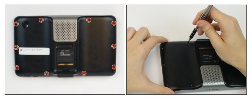
• Using a Torx T6 Screwdriver, remove the ten 7mm screws from the back panel.
