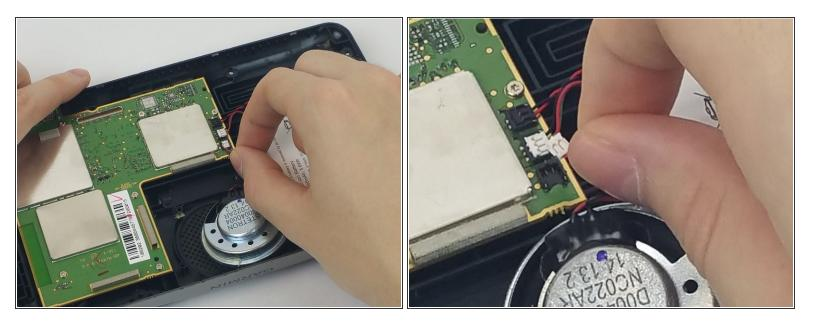
• Grasp the speaker wire near the motherboard and lift upward to detach the connector.
