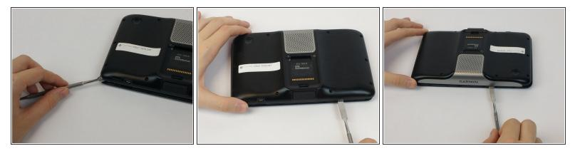
• Using a metal spudger, pry the device apart.
