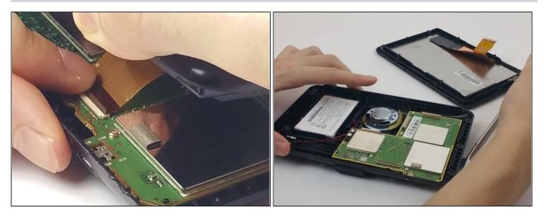
• Find and lift the small grey hinge at the end of the ribbon cable.
