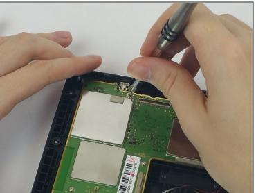
Using a Torx T5 screwdriver, unscrew the six 5mm screws on the motherboard.
