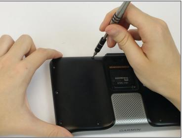
Using a Torx T6 Screwdriver, remove the ten 7mm screws from the back panel.
