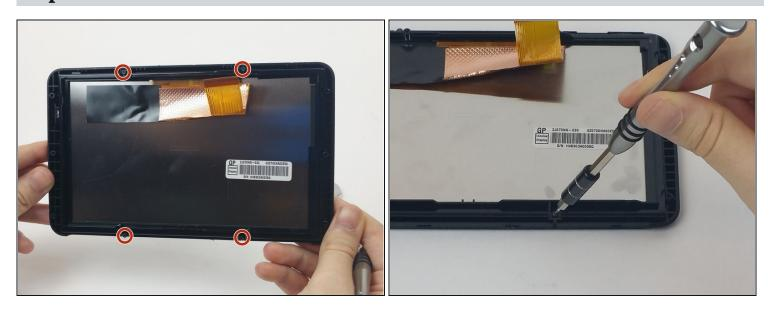
• Using a Torx T5 screwdriver, unscrew the four 7mm screws from the back plate of the screen.
