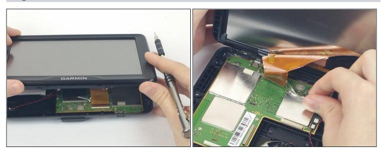
• Lift the screen opposite where the "GARMIN" logo is located. Remove the clear tape holding the ribbon cable to the motherboard.
