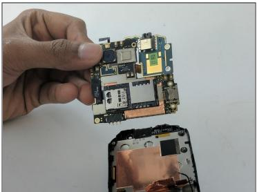
Carefully pull the motherboard out of its recess.
