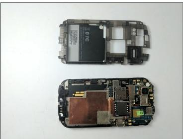
• Now simply remove the back panel by gently pulling. This will make it easier to access the devices internal components.
