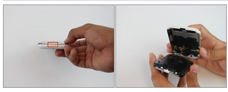
Gently press the Release Button located at the bottom of the phone in order to remove the back panel of the device.
