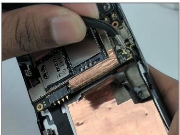
• Remove the power supply from the motherboard by gently pulling the end of the black wire with the precision <u>tweezers</u>.
