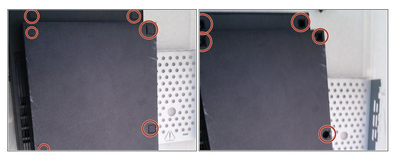
• first what you need to to do is take all the plastics of the bottom of the device which will reveal the screws.
