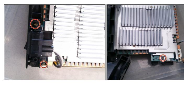
now unscrew the 2 copper screws to be able to make the bottom case will come out reveling a copper screw
