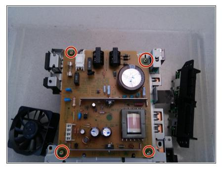
now flip the device to reveal the bottom. Now as soon as you flip you'll see 4 more copper screws, then your going to need to unscrew them unlocking the motherboard.
