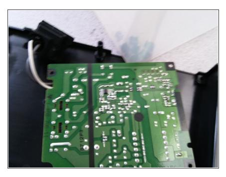
slowly pluck out the motherboard without braking no ribbons form the device. And that's how you take the motherboard out.
