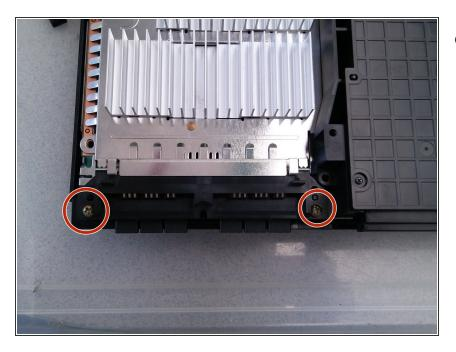
Once you've open the device you'll see 4 copper screws. Unscrew the front screws to unlock the bottom case of the device.
