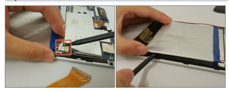
⚠ Make sure to not bend or puncture the battery when removing it.
