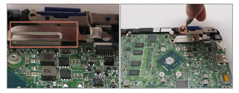
• Use the phillips screwdriver with the PH00 head to unscrew the one 3mm screw. Then, remove the bracket.
