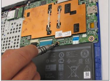
Use a Phillips screwdriver to unscrew the three 4 mm screws securing the battery.
