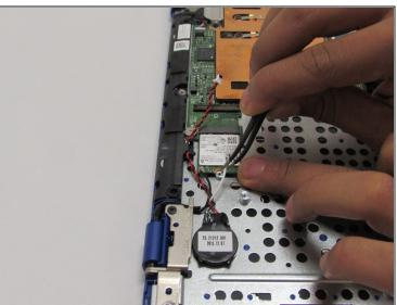
• Using the <u>tweezers</u>, pull the white and black wires off of the WiFi Chip.
