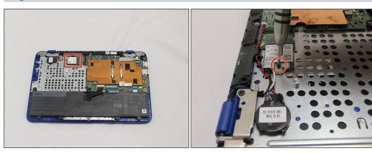
• Use the phillips screwdriver with the PH000 head to unscrew the 3.8mm screw.
