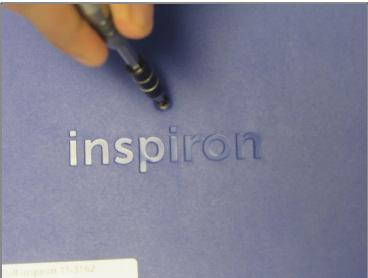
• Use a Phillips screwdriver to unscrew the nine 6.8 mm screws securing the back cover.
