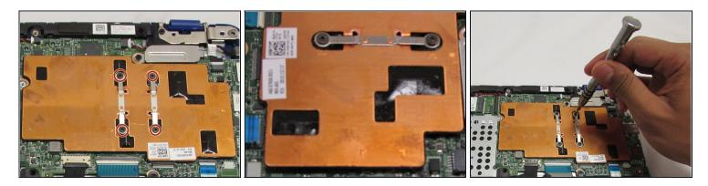
• Use the phillips screwdriver with the PH0 to loosen the 4 screws and remove the orange plate.
