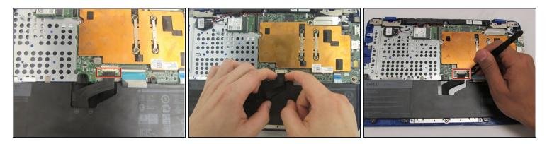
• Use your fingers (or a set of <u>tweezers</u>) to disconnect the battery cable from the motherboard by gently pulling it towards the battery.
