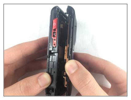
• Separate the front and back casing.
