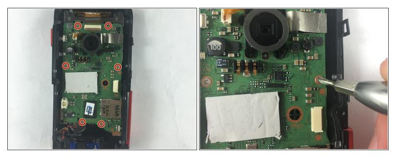
• Remove the six 2.00mm screws with Phillips #00 screwdriver.
