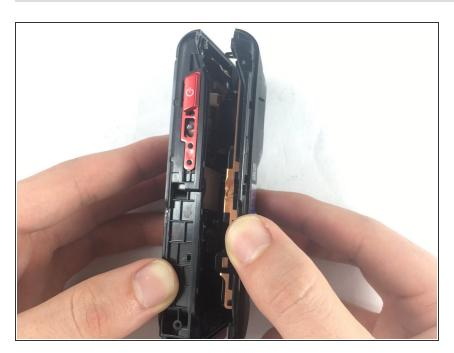
Separate the front and back casing.
