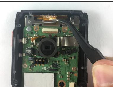
Use precision tweezers to remove the connector joining the LCD and the motherboard.
