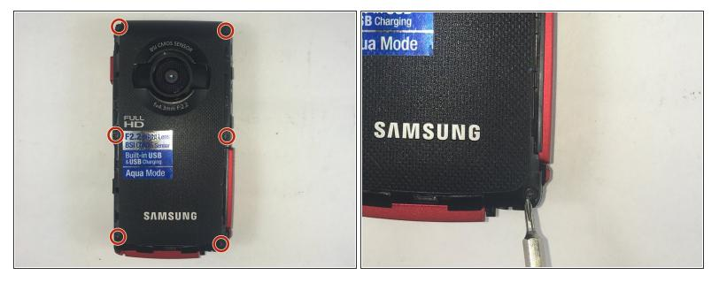
Remove the six 5.00mm screws by using a Phillips #00 screwdriver.
