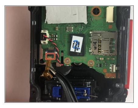
Use precision tweezers to gently pull out the USB connection from the motherboard.
