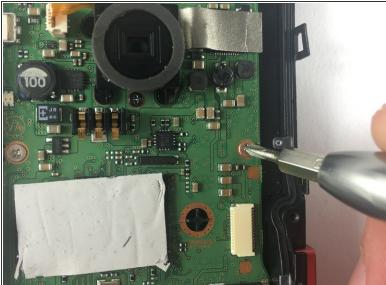
Remove the six 2.00mm screws with Phillips #00 screwdriver.
