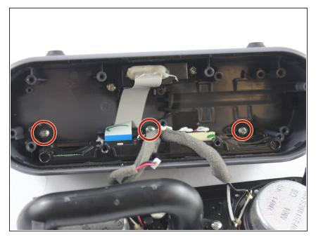
Use PH1 screwdriver to remove three 11mm Phillips head screws that are holding the motherboard together.
