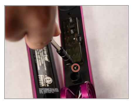
Using Philips head (PH1) remove the two 4 mm silver screws on the sides of dial panel cover
