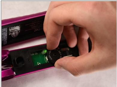
Using Philips head (PH00) to remove the 4 mm silver screw on the dial. Remove the dial with your hand.
