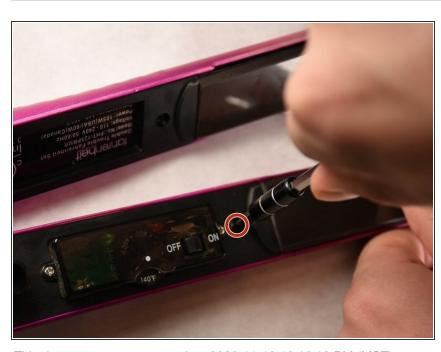
Using Philips head (PH1) remove the 6 mm black screw that was underneath the spring as well as the 6 mm black screw next to the heating plate. Remove the panel the screws were holding down.
