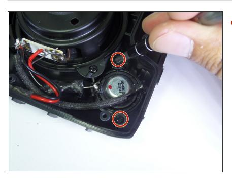
Remove the two 7.0 mm screws Phillips #2.
