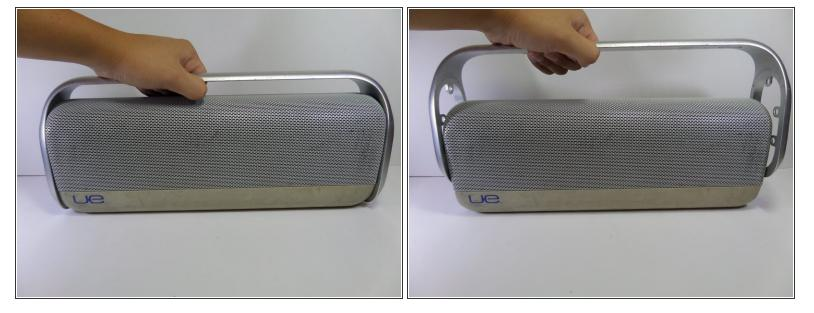
Pull up on the aluminum boombox handle to remove.
