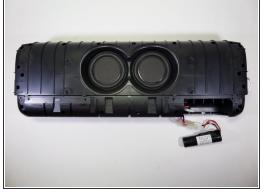
Pull vertically on the speaker grille to remove it from the boombox.
