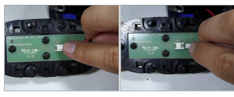
Firmly press on the end of the latch and pull the two-wire connector away from the base.
