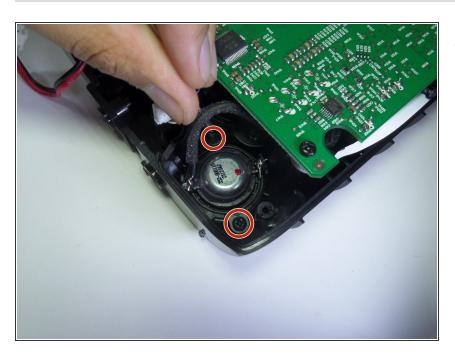
Remove the two 7.0 mm screws with a Phillips #2.
