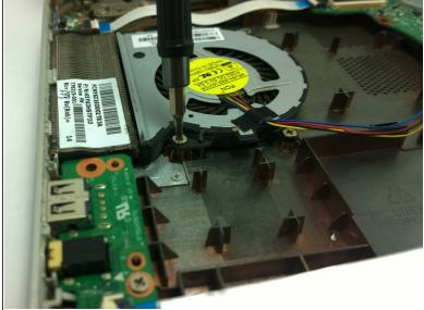
Remove the three 4.5 mm Phillips #0 screws holding the fan in place.
