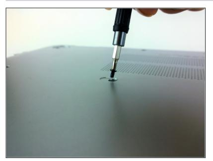
Remove the two cover tabs towards center of the bottom as there are screws underneath them.
