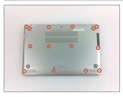
Remove all fourteen 4.5 mm screws from the bottom using a Phillips #0 screwdriver. Each location is marked by a red circle in the picture.
