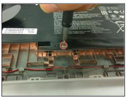
• Remove the three 3 mm screws from the battery using Phillips #0 screwdriver.
