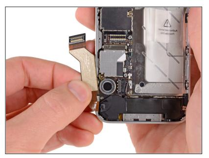
Peel the dock connector cable off the adhesive securing it to the logic board and the side of the speaker enclosure.
