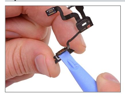
Use the edge of a plastic opening tool to separate the power button contact from its plastic bracket.
