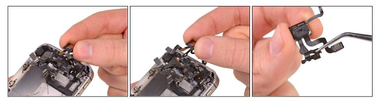
• Lift and remove the power and sensor cable assembly from the iPhone.
