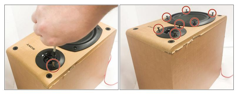
Remove the seven 18.06mm PH1 screws.
