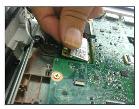
Gently remove the card from its slot by pulling.
