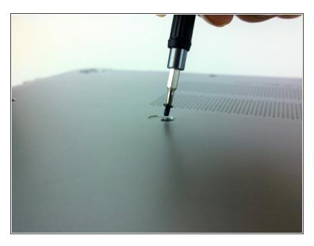
Remove the two cover tabs towards center of the bottom as there are screws underneath them.
