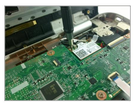
Remove the Phillips #0 4.5 mm screw from the wireless network card located in the back, right side of the interior.
