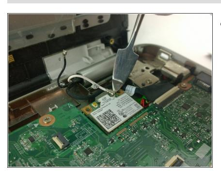
Detach the antenna connector for the white wire labeled "2".
