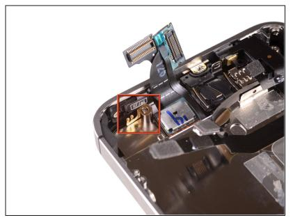
⚠ Be sure not to lose the small grounding finger for the rear facing camera near the power button. This finger rests on top of the PCB, screwed down, and covered with the adhesive black plastic tape.
