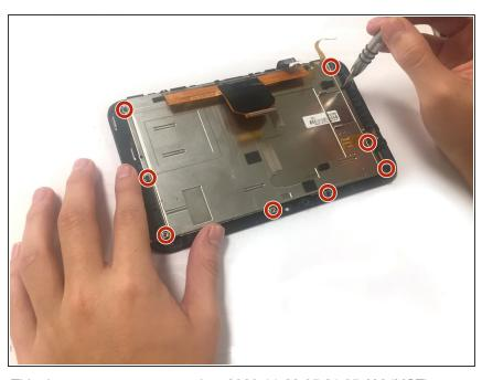
Using the screwdriver, remove the 3mm Torx T5 screws around the metal housing.
