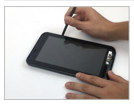
Use the spudger to go along the edges of the device and pop out the latches securing the display to the case.
