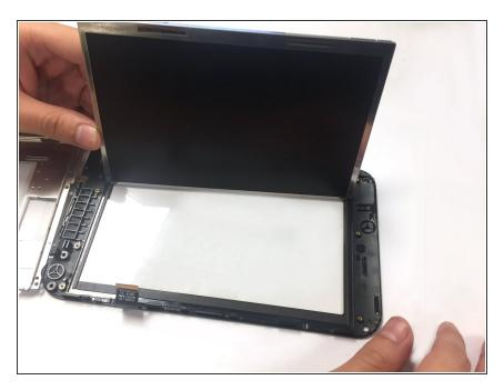
Remove the screen by lifting the screen from the front glass.
