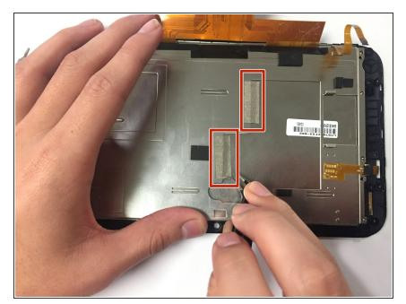
Using tweezers, peel off the tape securing the screen to the metal cage around it.
