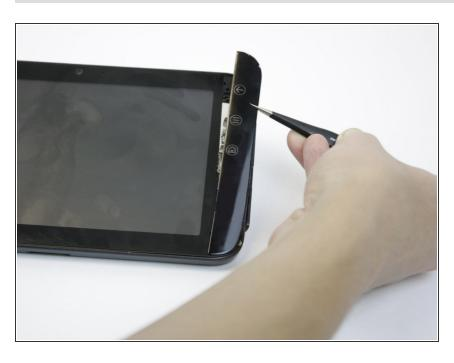
Remove the button cover by lifting the cover away from the tablet.
