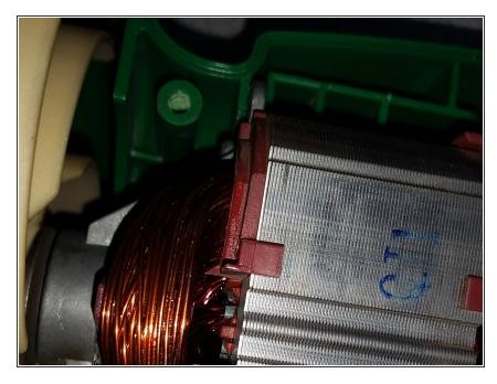
clean the dust out if you need to. then carefully put the motor back in making sure you put both of the tabs on the motor into their respective slots. you can't see the other one because I had to crop it out.
