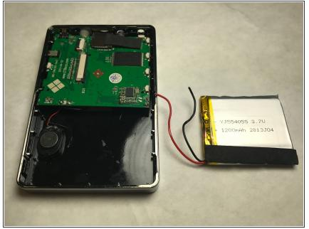
(i) You will have to clean the connections and solder the new battery back into place. Just as before, you want to reconnect the new battery to the motherboard.
