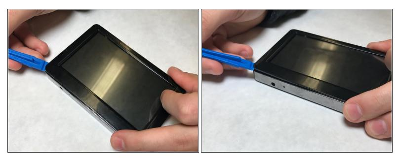
• Carefully pry up one of the top corners of the screen with a plastic spudger (prying tool). Slide the tool along the edges to release it from the housing.
