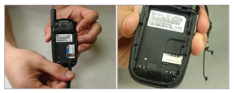
• Remove the sim card by sliding the card out from under the retainer using either your fingers or a spudger.
