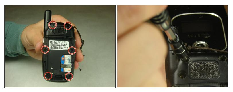
Remove the six 3mm #000 flat Phillips head screws from the back of the phone using a Phillips #000 Screwdriver.
