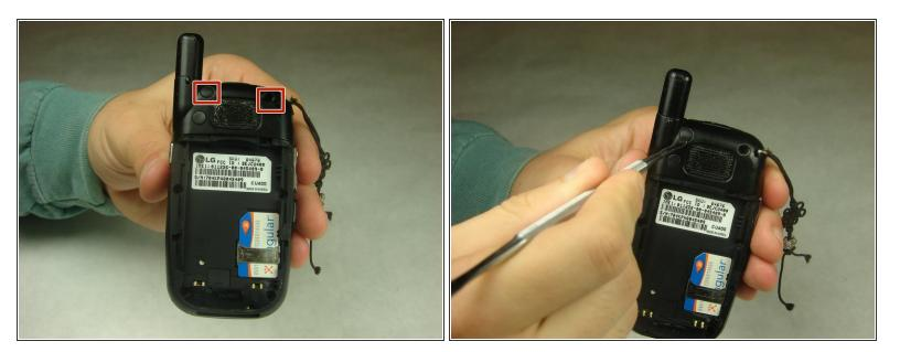
• Remove the rubber covers in the highlighted locations using a metal spudger.
