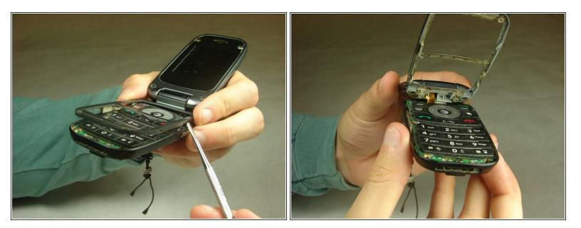
Once you have worked your way around the perimeter of the phone, you will have access to the components in the bottom half assembly.
