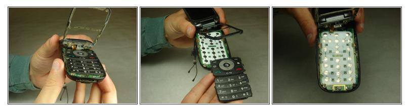
• You should notice that the number pad is loose and can simply be taken out of the open phone casing.
