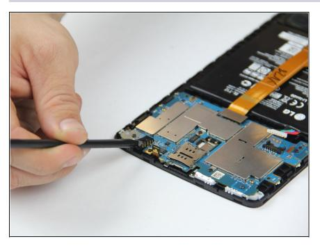
Pry the audio jack from the device using a spudger.
