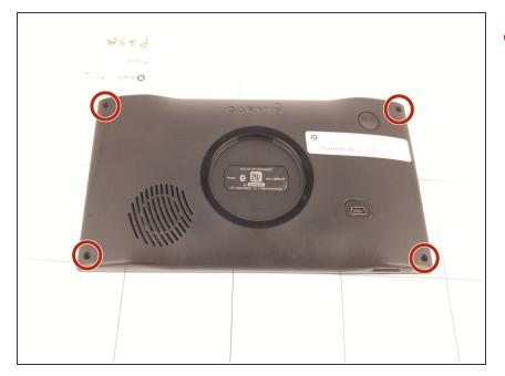
Remove the four 4mm hex screws from the four corners of the unit using a T5 bit.
