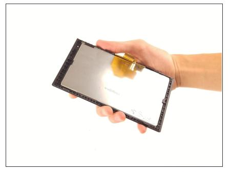
• Retrieve a new screen and connect the flat-gold wire to the socket from where you removed the old screen.
