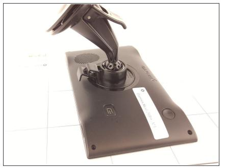
Remove the stand by depressing the tab and rocking the round interface back away from the tab, pulling it away from the Garmin unit.
