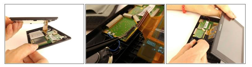
• Do not attempt to separate the unit until all the tabs have been separated. Once the seam is completely separated, you can lift the back away from the screen easily.
