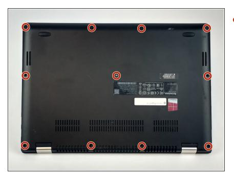
Remove the eleven 6mm T5 Torx screws from the back case.
