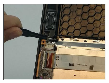
Using a pair of tweezers, dissconnect the speakers on the left side of the laptop.
