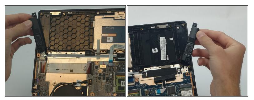
Both speakers are held in place by plastic pegs. Gently lift the speakers off the casing to remove them.
