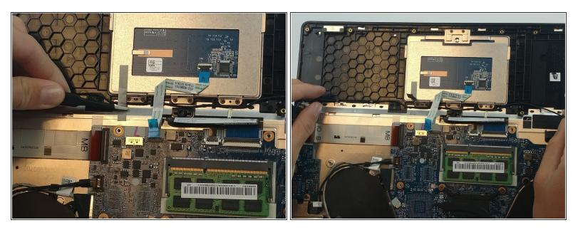
Use tweezers to gently pull off tape that is holding down wires that are connecting the two speakers together.
