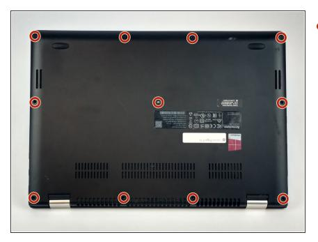
Remove the eleven 6mm T5 Torx screws from the back case.
