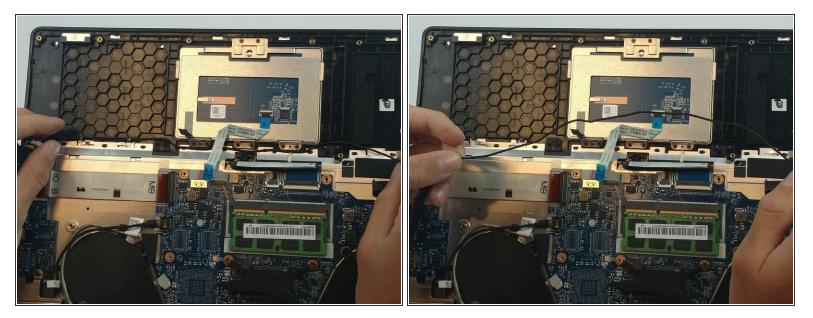
• Simply grip the speaker wires and lift away from laptop to remove.
