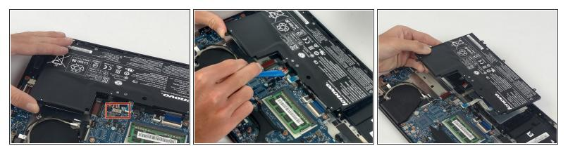
• Gently lift the battery and use the plastic opening tool to remove the battery's connection to the laptop.
