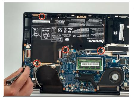
Remove the four 3mm PH#0 screws surrounding the battery.
