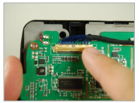
Remove the bottom LCD connector by gently pulling it away from the motherboard.
