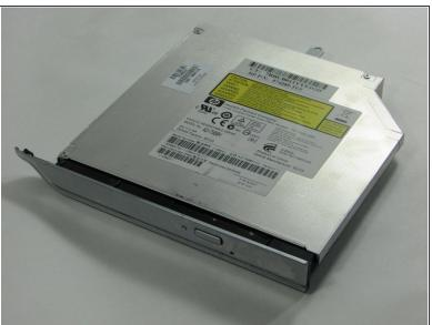
Gently pull the Optical drive out of the slot until the whole thing comes out.
