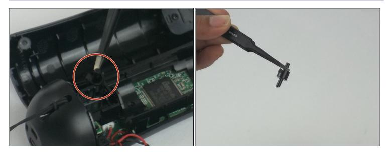
• Using <u>tweezers</u>, remove the small piece with a cylindrical top that is located to the left of the inner plastic frame.
