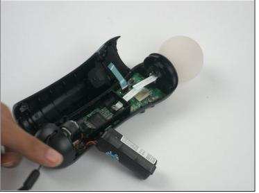
• Once the device is opened, lift the battery out of the black plastic holder.
