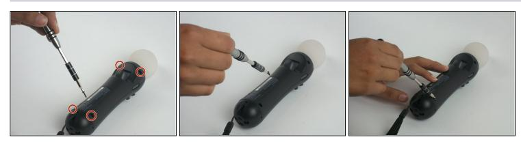
Using a Phillips #0 screwdriver, remove the four 10mm screws located on the back of the device.
