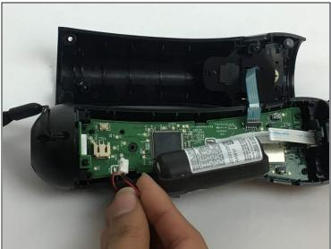
• Gently pull on the white piece connecting the battery and the connector.
