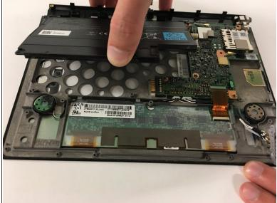
• Use the spudger to pop the battery loose and remove the battery.
