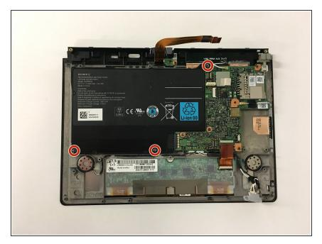
Remove the three 5mm Phillips #0 screws securing the original battery.
