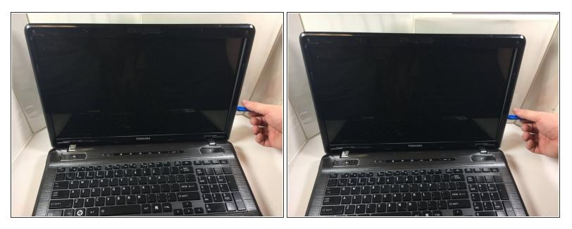
• Gently remove the plastic lining of the screen. Use a card, guitar pic, or another tool to pry open the lining, but be careful during this process.
