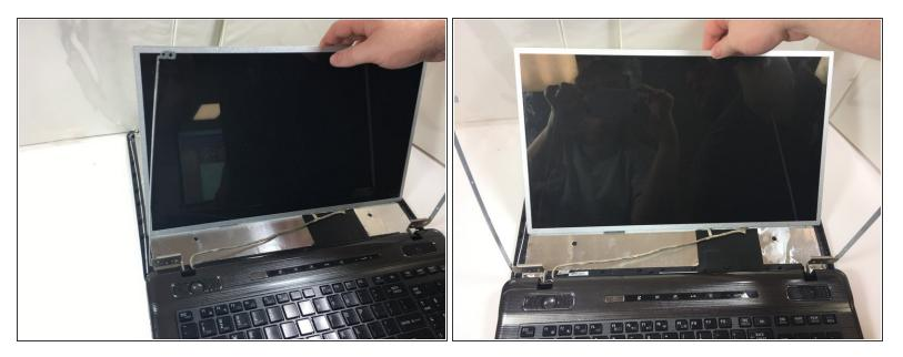
At this point, your screen is almost disconnected. Be sure to support the screen because there is nothing holding it up.
