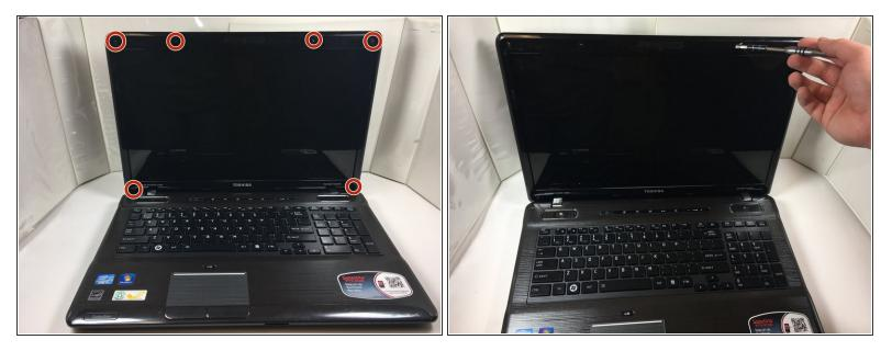
Begin by removing all of the screws around the perimeter of the screen. There are 6 total.
