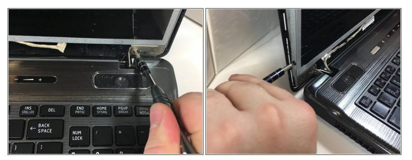
Unscrew the screws located on the sides of the silver part of the screen. Some of the screws are smaller than others, so be sure to get all of them. The screen cannot come off if the screws are not all out.
