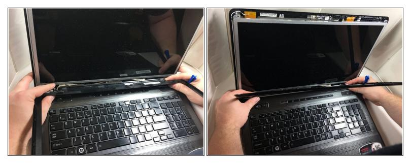
Once the plastic lining is loose from the device, you can remove the lining. Gently pop the lining of the screen off of the hinges of the computer.
