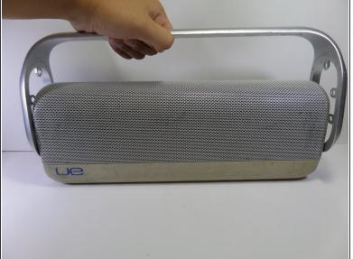
Pull up on the aluminum boombox handle to remove.
