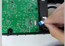
• Pull up on the lock to detach the band connector from the motherboard.
