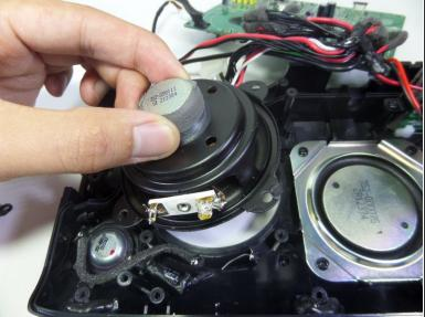
Lift the speaker out of the device using your fingers.
