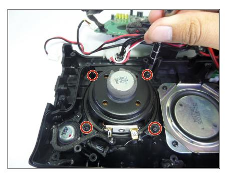
Remove four 7.0 mm screws with a Phillips #2.
