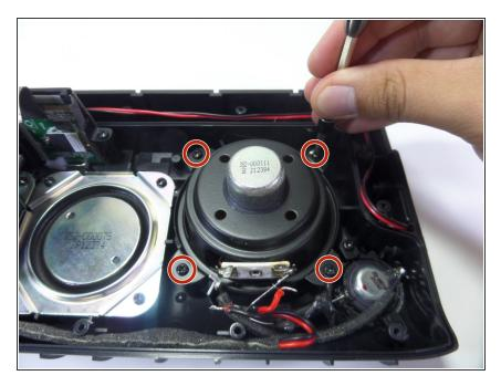
Remove the four 7.0 mm screws with a Phillips #2.
