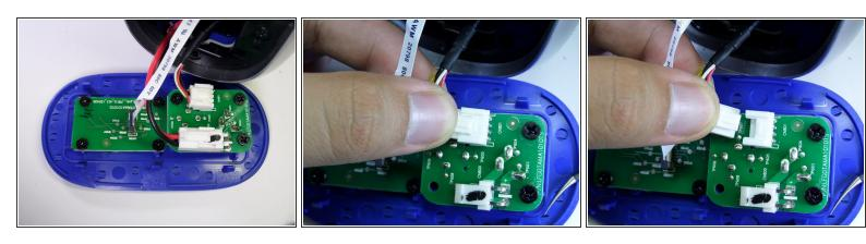
Firmly press on the end of the latch and pull the four-wire connector away from the base to separate.
