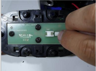
Firmly press on the end of the latch and pull the two-wire connector away from the base.
