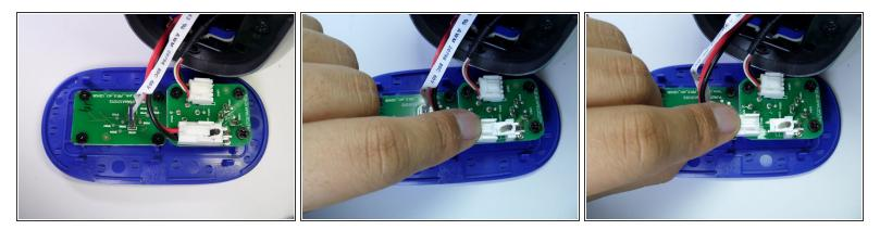
Press firmly on the end of the latch and pull the two-wire connector away from the base to separate.
