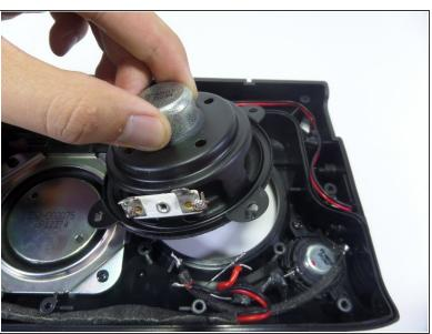
Lift the speaker out of the device using your fingers.
