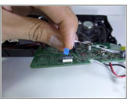
Pull up on the lock of the band connector to detach it from the motherboard.
