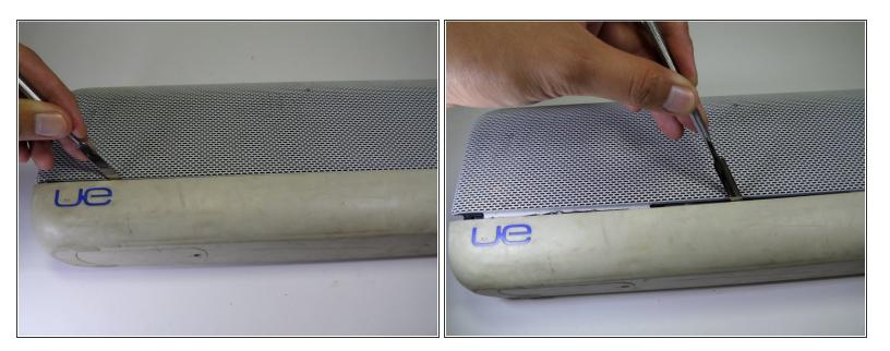
Use a metal spudger to pry the rubber base apart from the aluminum grille.
